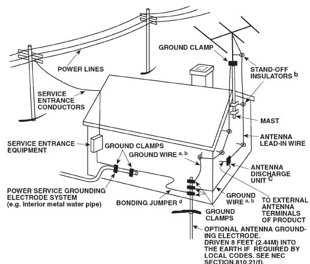
**NOTE TO CATV SYSTEM INSTALLER:** This reminder is provided to call the CATV system installer's attention to Article 820-40 of the National Electrical Code that provides guidelines for proper grounding and, in particular, specifies that the ground cable ground shall be connected to the grounding system of the building, as close to the point of cable entry as practical.
